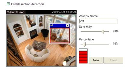
The Percentage Indicator will rise or fall depending on the image variation. When motions are detected by the Network Camera and are judged to exceed the defined threshold, a red bar rises. Meanwhile, the motion detection window will be outlined in red. Photos or videos can be captured instantly and configured to send to the remote server (Email, FTP) by utilizing this feature as a trigger source. For more information about how to plot an event, please refer to Application on page 60.
